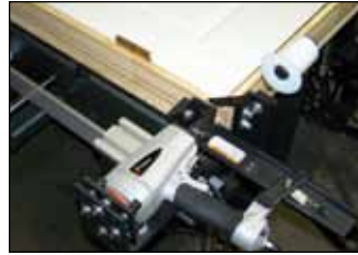
Jambs are securely clamped during stapling.
