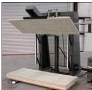
Doors are individually picked from a stack to reduce damage.
