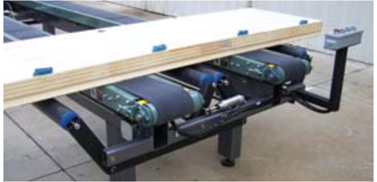
Dual belt conveyors and pop up rollers
