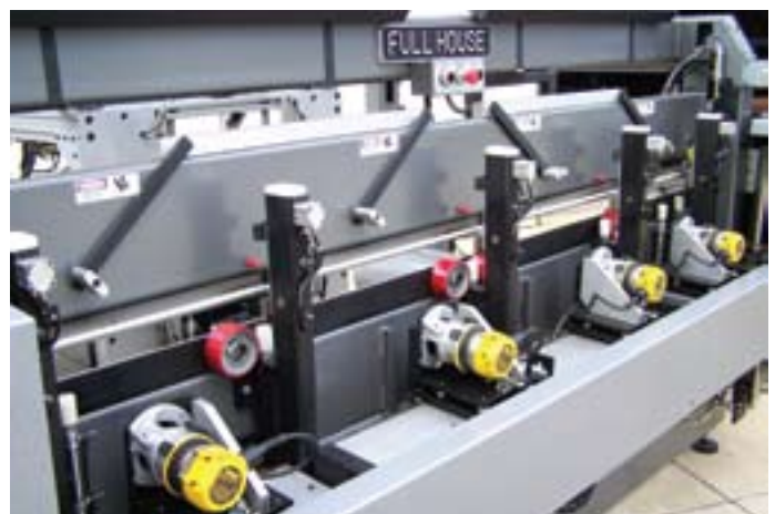
Automatic Hinge Routing
