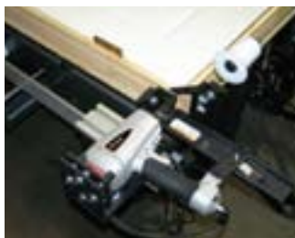
Jambs are securely clamped during stapling.
