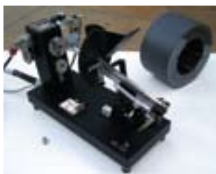
Quick change bowl for switching screw colors
